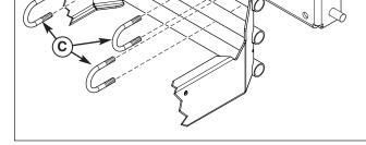
Figure 2. Install Hitch Plate (Tube Style Bumper)
